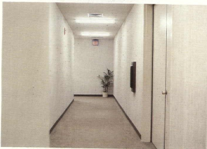
The corridor serves as a transition space between the relatively dark simulator and the brighter classroom and learning center spaces. In the renovated space, corridor illuminance is only 5 footcandles; previously, average illuminance on the floor was 50 footcandles.
