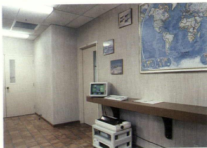
Student contact with the center begins at the computer check-in and check-out station. Before the lighting-only renovation project, the area was overlighted by glaring, wraparound fluorescent luminaires.
