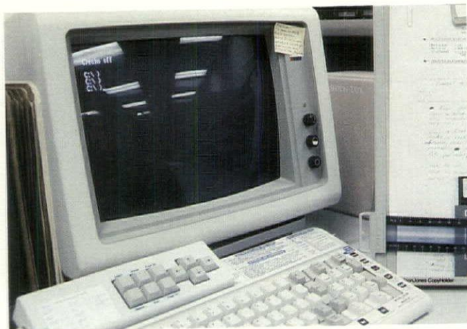
Before the renovation, VDT screens in the instructors' office mirrored the lensed 2 x 4 luminaires.
