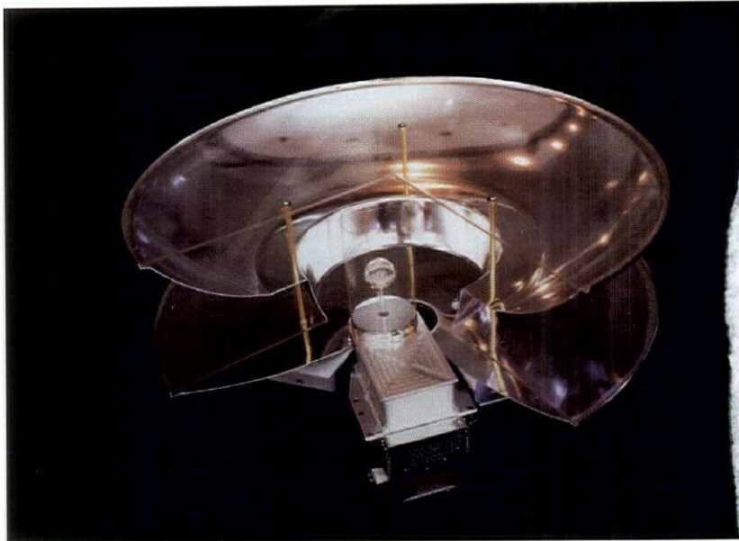
THE COOPER LIGHTING FIXTURE. SPECIAL OPTICS HAD TO BE DESIGNED IN A PARTNERSHIP WITH SCIENTISTS AT THE LAWRENCE BERKELEY LAB TO ACCOMMODATE THE UNIQUE PHYSICAL AND ILLUMINATING CHARACTERISTICS OF THE SULFUR LAMP.
