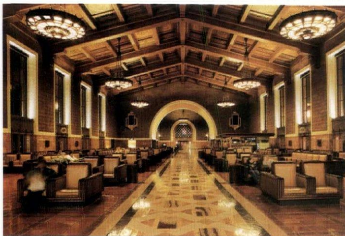
OPPOSITE: SODIUM VAPOR FLOODLIGHTS BATHE THE FRONT FACADE IN AN AMBER LIGHT. THE WARMER TONES RESONATE AGAINST THE COOL HUES OF BLUE FILAMENT METAL HALIDE SOURCES. INSIDE THE MAIN WAITING ROOM (ABOVE), SPOTLIGHTS ILLUMINATE THE WINDOWS AND UPLIGHT THE CEILING TO BRIGHTEN THE SPACE.
