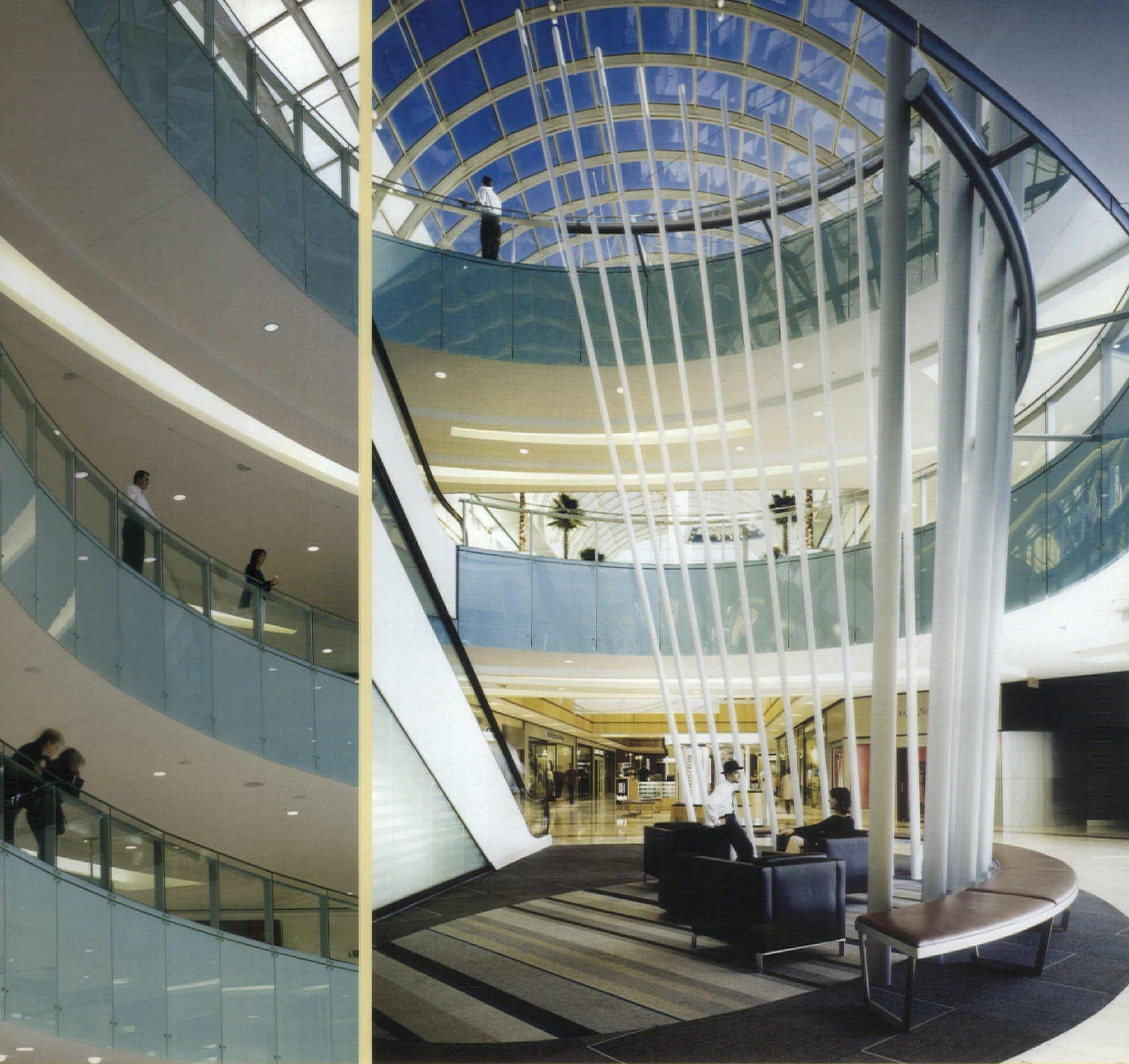
PAR30 metal halide recessed downlights and fluorescent cove lights define the ceiling planes of the main circulation corridors (center). Equally spaced, canted poles provide semi-private seating areas, and add vertical dimension to the elliptical-shaped circulation nodes (top right).
