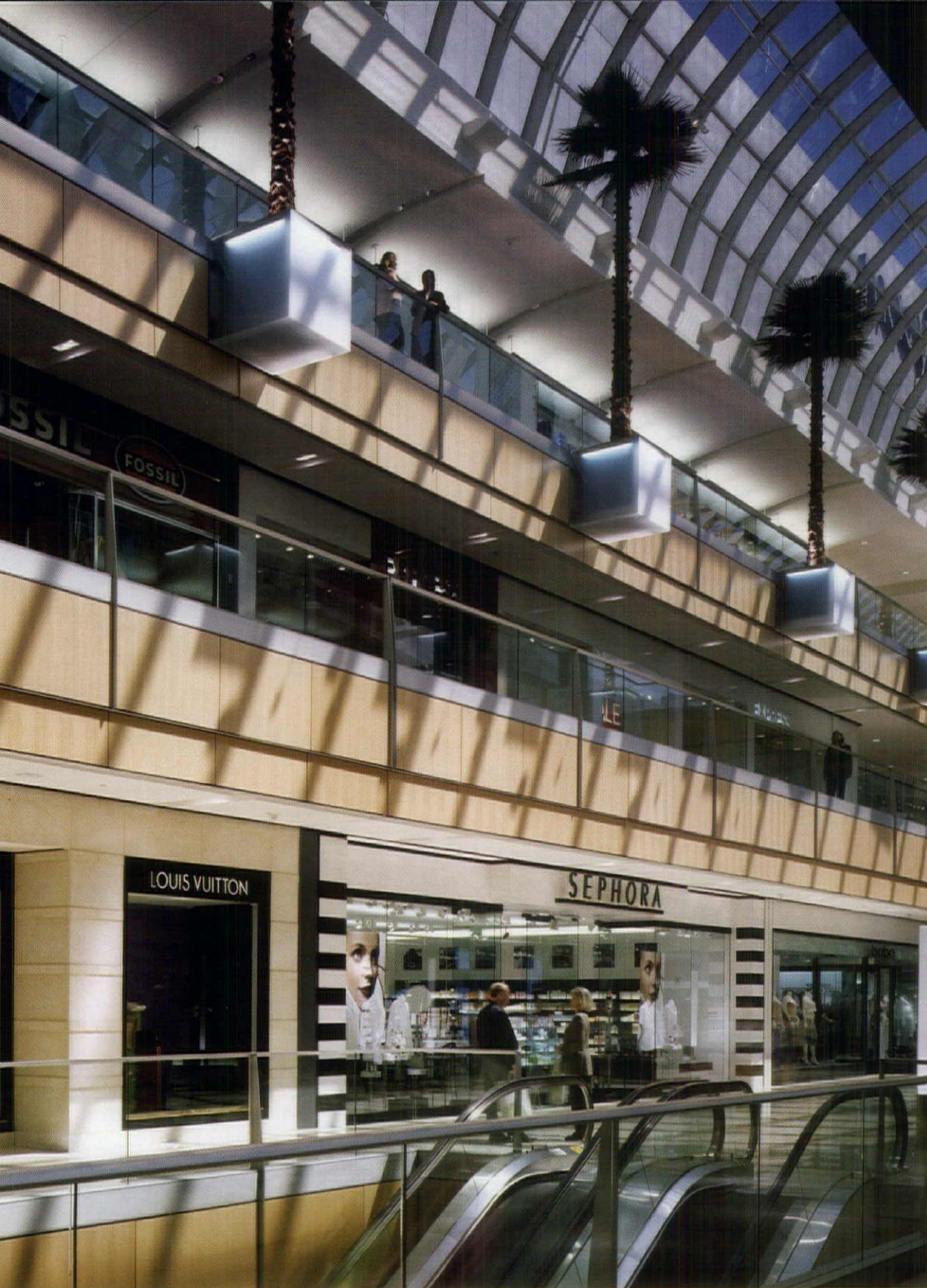
A neutral palette of eucalyptus wood panels and transparent and back-painted glass railings provide additional reflective surfaces for the distribution of daylight. Indirect fluorescent luminaires uplight the underside of the third-floor corridor soffit (above). The new finishes also remedied the dated color scheme of the original interiors (top and bottom right).
