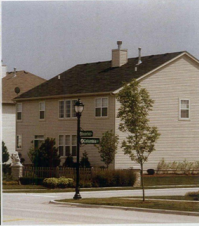
Mounting height is critical. Pedestrian-scale lighting, for example, does not effectively light the roadway and looks out of proportion with the scene.
