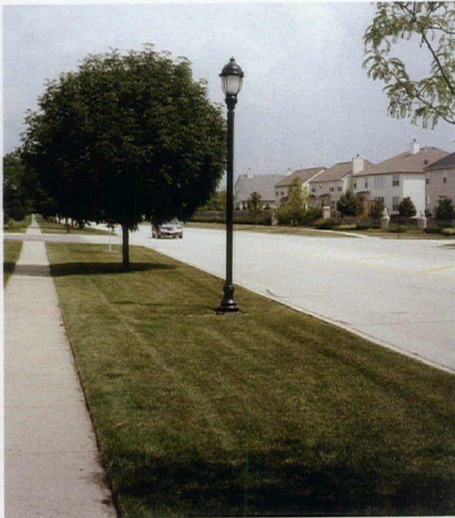
Mounting height is critical. Pedestrian-scale lighting, for example, does not effectively light the roadway and looks out of proportion with the scene.
