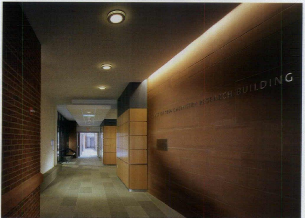
The Yale Chemistry Research Building integrated daylighting and electric lighting systems to optimize lighting quality and energy efficiency (above). The second level lounge is indirectly lighted to supplement the available daylight (below).
