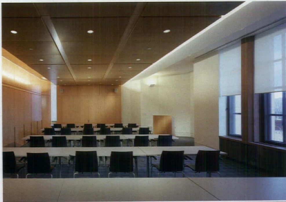
The conference room uses dimmable fluorescent ambient and halogen accent lighting on programmable controls (above).
