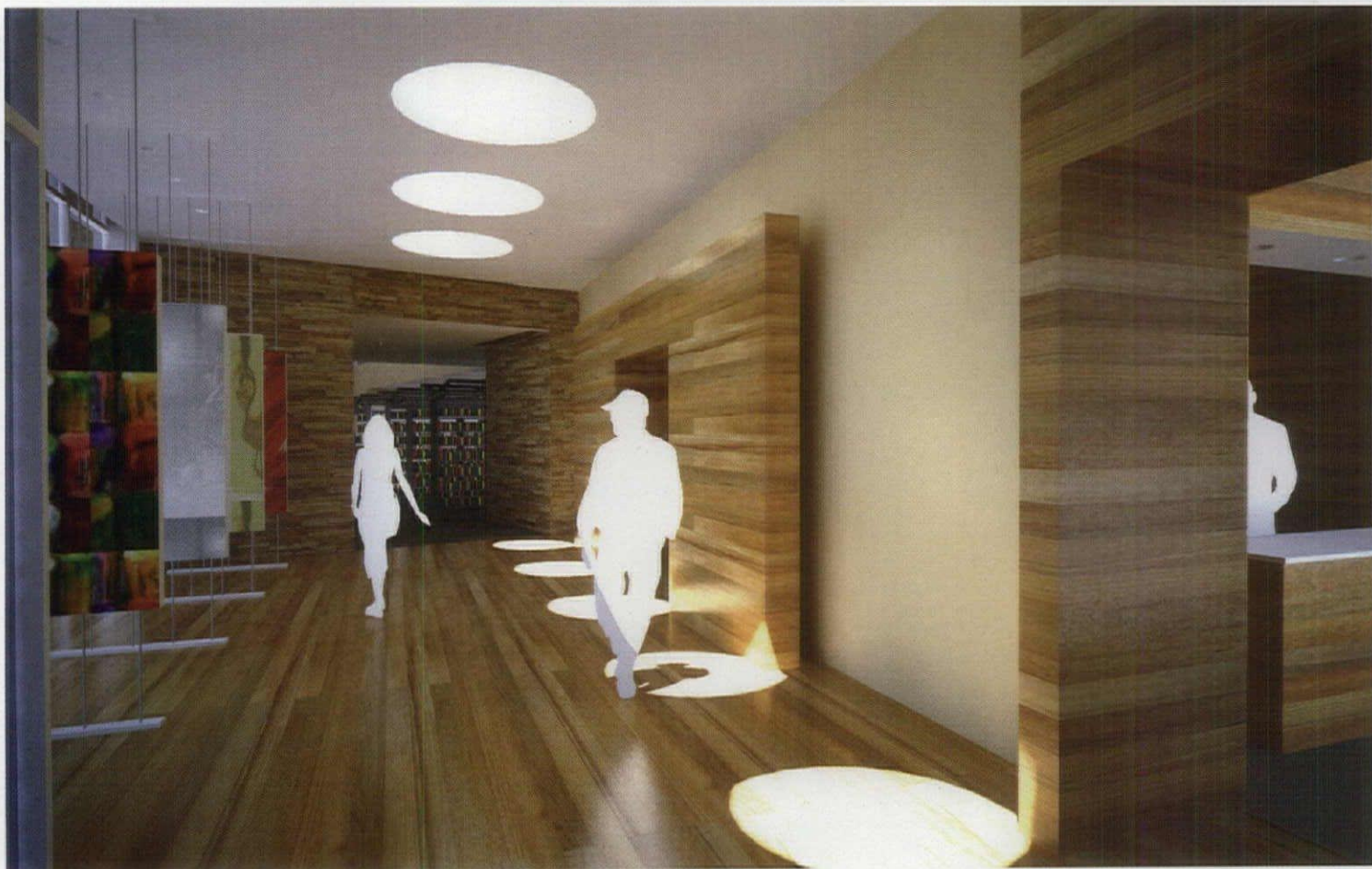
Using AGi32, a software tool for daylight and electric light simulation, Team NaCK rendered its building so it could better understand how its architectural decisions were impacting their lighting choices. Here is a view of the entry area (above), the library stacks (right), and the entrance and public plaza (bottom right).
