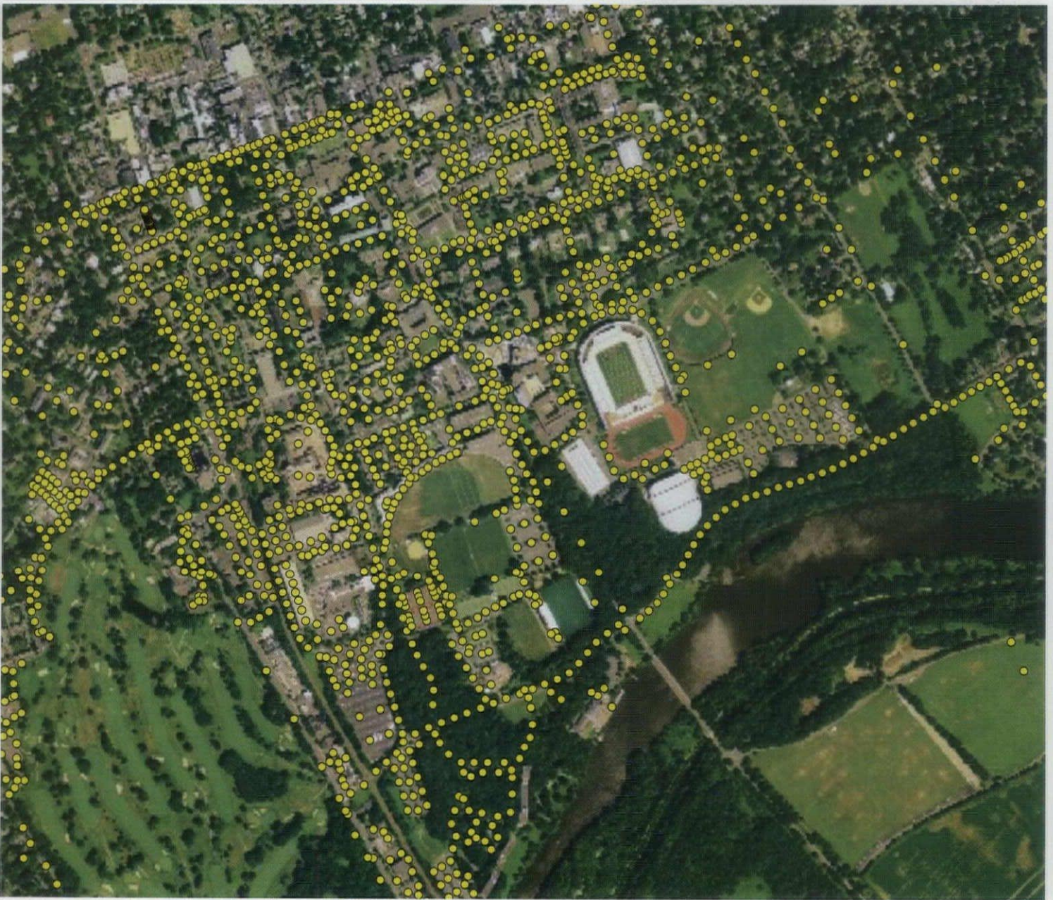
The Princeton Exterior Pathways project analyzed Princeton University's existing lighting conditions—all 1,720 exterior pathway luminaires (above)—and created a numbering system for the facilities department to use for day-to-day operations. Under the guidance of faculty member Paul Lewis, the team of student researchers—graduate architecture students Jean Choi, Yu-Cheng Koh, and Thomas Wong (top)—spent eight weeks from June to August this past summer conducting field research and mapping light levels. For this, they created a machine they named the Luxmetron (left)—a mobile light measuring device that they rolled across campus and from which they compiled 10,986 readings for their lighting analysis.
