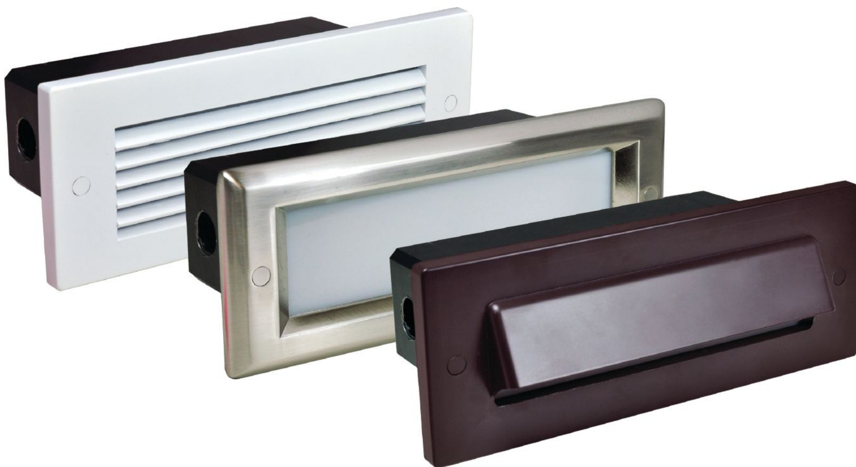
LED Brick Step Lights, Nora Lighting • Designed to be the size of a standard brick (8 5 / 8 " by 3 15 / 16 " by 3" deep), the LED Brick Step Lights were designed for pathway and step lighting. Each fixture has 24 4W LEDs and is available in 2925K. The die-cast aluminum faceplates can be specified as louvered, lensed, or shroud. Finish options are brushed nickel, bronze, and white. • norlighting.com • Circle 294
