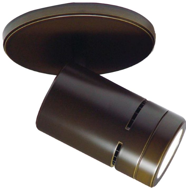
LED Monopoint, No. 8 Lighting • Part of the Beyond Halogen LED family of luminaires, the LED Monopoint is Title 24 compliant. It uses Philips' Lumileds Luxeon S LED with an 85 CRI, 3000K, 1,050-lumen light engine. The fixture is ceiling- and wall-mountable and the fixture head can adjust up to 320 degrees and tilt up to 100 degrees. The all-aluminum housing has four finish options: white, black, oil-rubbed bronze, and satin aluminum. UL listed for damp locations. • 8lighting.com • Circle 130
