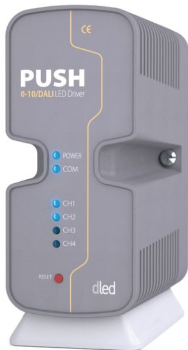
Push, d-LED • Push is a four-channel constant-current LED driver that enables high-power LED lighting applications of up to 48 (4x12) LEDs. It measures 4.7" deep by 4.1" wide by 7.3" tall and can be installed on either Din-Rail or directly on structure. It can be controlled by DALI protocol, zero-to-10V, or DMX-512 signals. It also has an active thermal protection feature. • d-led.net • Circle 345
