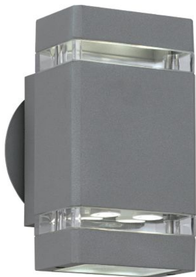
Possini Euro Design Matte Silver Gray LED Outdoor Wall Light, Lamps Plus • The Possini Euro Design Matte Silver Gray LED Outdoor Wall Light comes with a matte silver-gray finish with clear glass and has both an uplight and a downlight component. It uses eight 1W LEDs, is available in 2900K to 3100K, and has a lumen output of 455. It is not dimmable. The luminaire measures 8" high by 4 1 / 4 " wide, and projects 4" from the wall. • lampsplus.com • Circle 291
