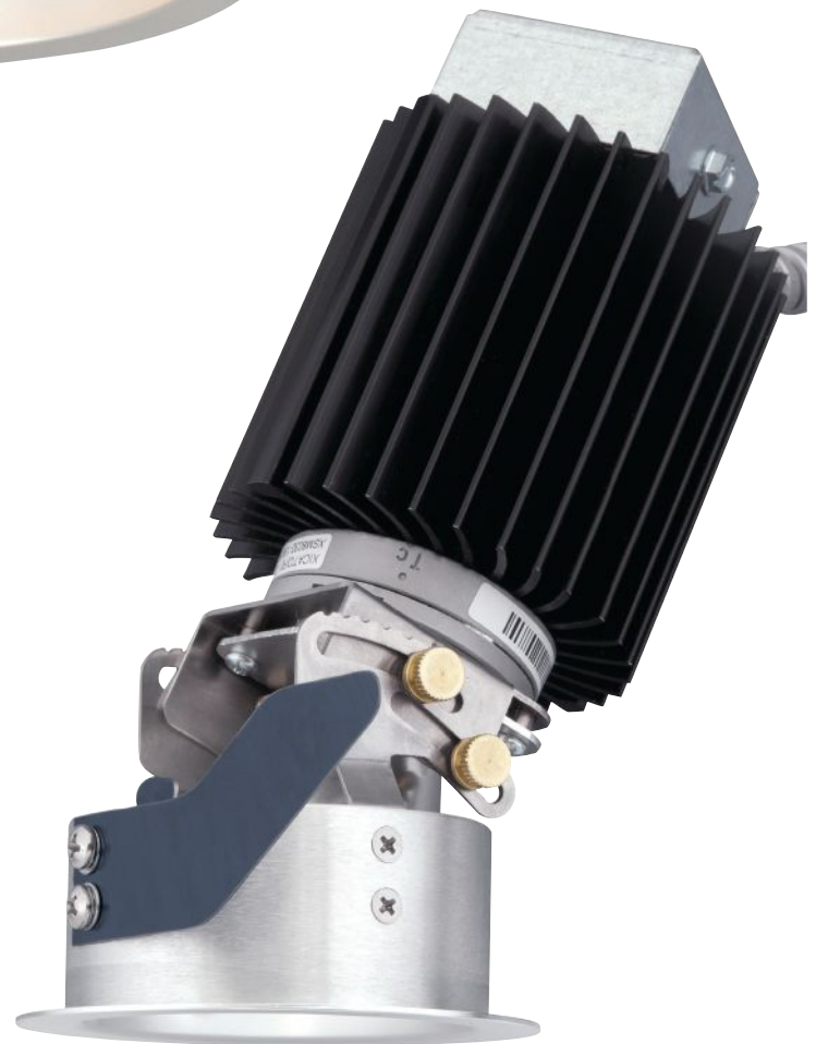
A2LED, Prescolite • Part of Prescolite's 2" LED series, the A2LED was designed to address sloped ceiling conditions as well as accent lighting applications. It uses Xicato's Artists Series LED module and has a 35-degree optical pattern that can be adjusted and locked up to 30 degrees from vertical. The luminaire is capable of 360-degree rotations and is compatible with new construction or retrofit installations. • prescolite.com • Circle 131
