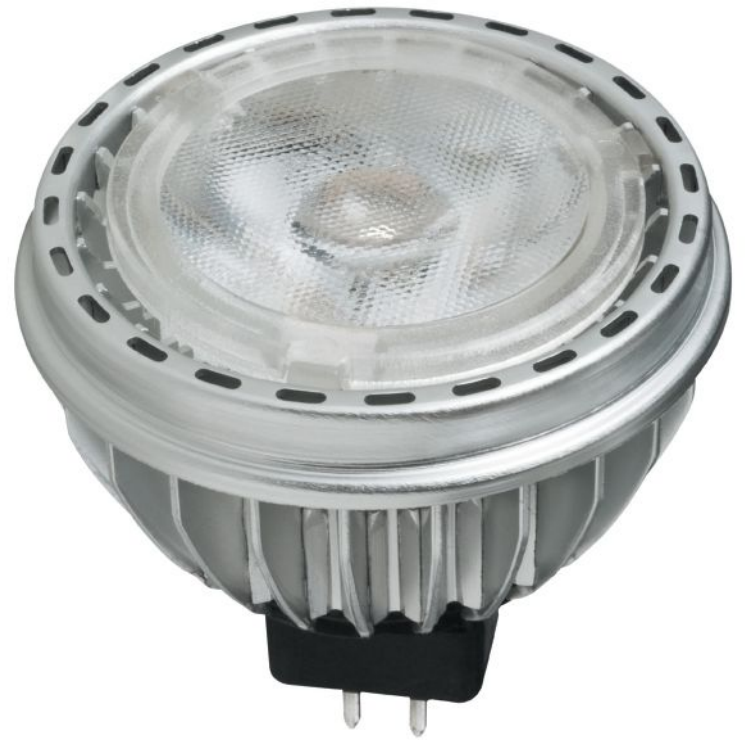
LM16 LED Replacement Lamp, Cree • Cree's LM16 LED Replacement Lamp is designed to take the place of a 50W halogen MR16 lamp. It works with a broad range of transformers and dimmers, delivers between 425 and 620 lumens, and has a color temperature of 3000K. The lamps are also available in a variety of beam angles (17-degree Spot, 25-degree Flood, and 40-degree Wide Flood.) It can be dimmed to 5%. • cree.com • Circle 323
