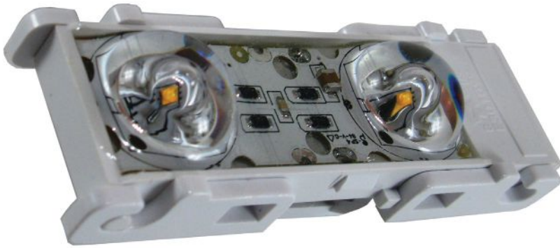
Polyoptik, Heico Lighting • Designed for architectural lighting applications, the 3500K Polyoptik LED modules are part of Heico's Contactless LED System and feature Narrow to Wide beam angles for uniform illumination. The modules are inserted on one electrical circuit connected to the LED master power supply, which has AC power conveyed by electromagnetic induction, eliminating electrical contacts and corrosion risk. • heicolighting.com • Circle 332
