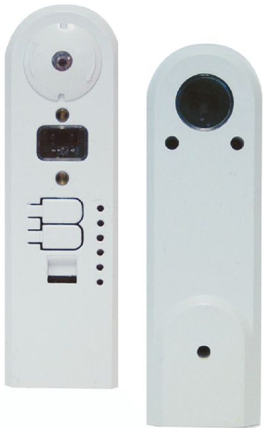
LMLS-600, WattStopper • The LMLS-600 is a dual-loop photosensor that provides daylighting control for applications with skylights. The device automatically switches or dims one zone of lighting based on ambient and daylight levels. An open-loop sensor detects daylight contribution while a closed-loop sensor reads the ambient light level. The LMLS-600 operates on Class 2 power. • wattstopper.com • Circle 328
