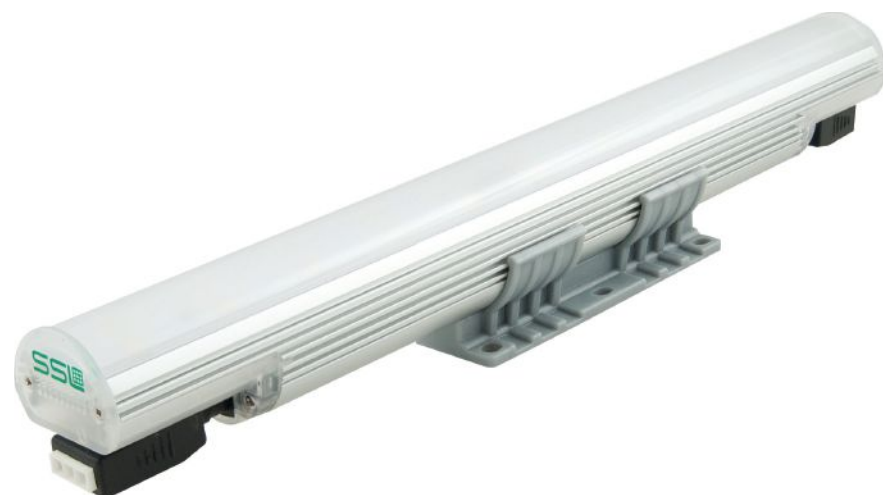
Coveline, FC Lighting This LED cove luminaire is available in 1', 2', and 4' nominal lengths and three color temperatures: 2600K, 3000K, and 4000K. It also has seven beam distributions: 25 degrees, 40 degrees, 60 degrees, 80 degrees, 120 degrees, 30 by 60 degrees, and 67 by 140 degrees. Its housing is constructed of extruded aluminum with tooled end-caps. The luminaire is rated for interior use only and features plug-and-play connectors to aid in installation. It is dimmable to 5% brightness. • solidstateluminaires.com • Circle 346
