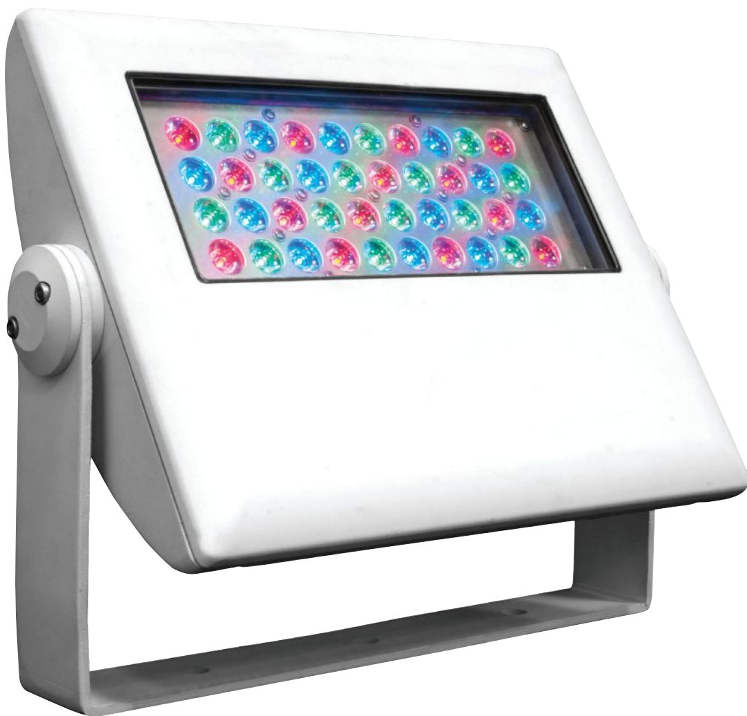
Illumipanel 40 IP, Illuminarc • This exterior washlight is designed to uplight walls, trees, or statues. It has 40 3W RGB LEDs and a 30-degree lens, as well as an impact-resistant glass cover. The luminaire also features built-in automated programs and 11 customizable color temperature presets. It measures 14.6" wide by 12" tall by 3.5" deep and runs on 100V or 240V AC power. • illuminarc.com • Circle 289
