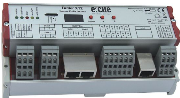
Butler XT2, Traxon e:cue • The Butler XT2 controls up to 1,024 DMX/RDM channels, is scalable up to 65,536 channels, and supports RDM protocol for bidirectional communication. The DMX/RDM engine can be used either in stand-alone mode to replay and loop lighting shows previously uploaded using e:cue's software suite on a PC, or it can be controlled by another of the company's engines. • traxontechnologies.com/us • Circle 335
