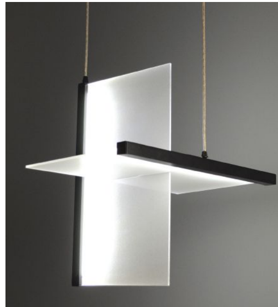
Planar 2D P-180 Series, DigitalSpeck Lighting • The Planar 2D Series pendant is part of Manning Lighting's new dedicated line of solid-state luminaires called DigitalSpeck Lighting. Six strips of 42W 4000K LEDs are integrated into two bisecting anodized aluminum planes that simultaneously serve as the heat sink. A proprietary microlens pattern evenly illuminates both sides of the extrusions and produces 4,410 total lumens. Each LED board is compatible with 120V or 277V electrical systems and zero-to-10V dimming equipment. • digitalspeck.com • Circle 119
