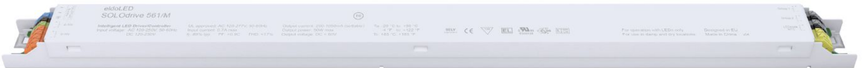
Solodrive 561/M, eldoLED • The Solodrive is a zero-to-10V dimmable, constant-current LED driver that offers smooth dimming all the way down to zero. It can be used for a variety of lighting applications including architectural, retail, signage, and street lighting. It offers two LED outputs to drive very high-power 50W LED arrays connected to a single output or two strings of 15 LEDs at 350mA. For use in dry and damp locations. • eldoled.com • Circle 334
