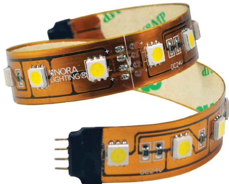
24V Hy-Brite, Nora Lighting • The 24V Hy-Brite LED tapelight can be used for a variety of applications including coves, undercabinet lighting, and backlighting. It has a maximum range length of 16' with magnetic dimmable drivers and a length of 32' with electronic drivers. It includes 2.7W (12 LEDs) per foot, comes in three color temperatures (2700K, 3000K, and 4200K), is dimmable, and is IP-44 rated for damp locations. • noraaighting.com • Circle 344
