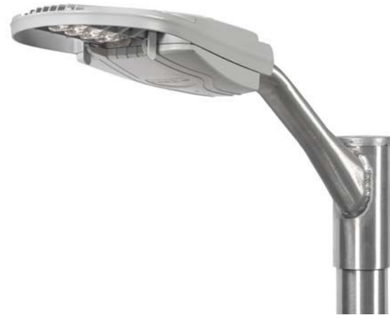
XSPR LED Residential Street Light, Cree • Cree designed this cobra-head-style LED street luminaire to replace high-pressure sodium fixtures in residential neighborhoods. The XSPR can be lamped with either a 42W or 25W LED source in 4000K and 5700K. A contemporary silver-finish, die-cast aluminum cover and horizontal tenon mounting system is adjustable to plus or minus 5 C. • cree.com • Circle 359
