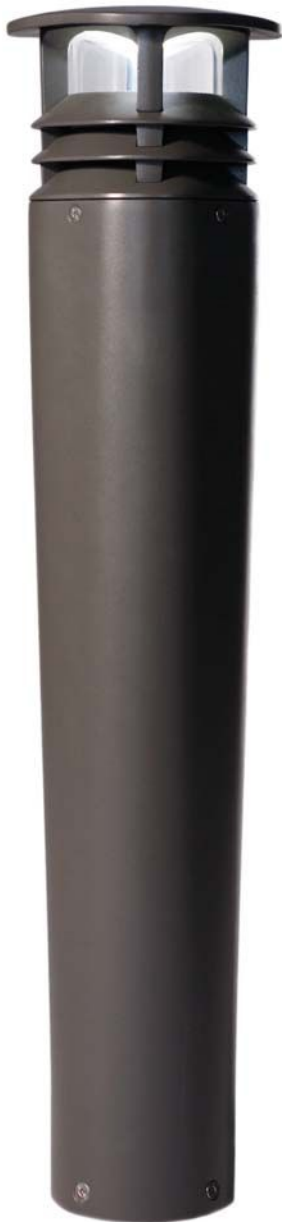
Cordia LED Bollard, Forms+Surfaces • Designed to coordinate with Cordia's family of benches and trash and recycling receptacles, this bollard has a powdercoated aluminum body available in a range of colors and with an optically clear acrylic lens that emits either 360-degree or 180-degree light. Measuring 38" tall, the fixture has an 8"-square top that tapers to a circular 6.38"-diameter base. Lamped with a 35W LED module, the luminaire is available in 3000K and 4000K. • forms-surfaces.com • Circle 360
