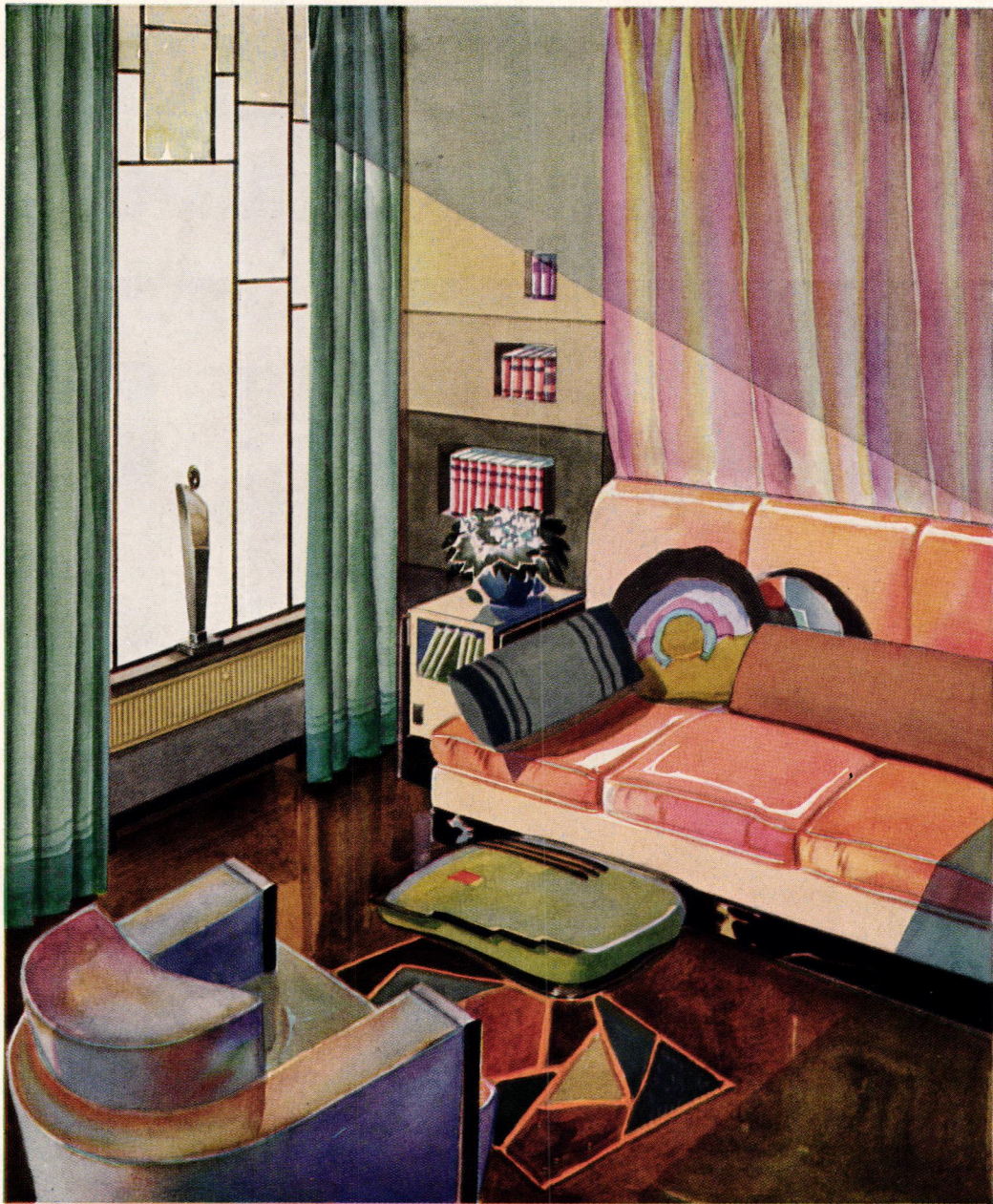
Radiator (1) comes installed in a steel case (2) more substantial than the wall itself. The complete unit is ready to install in any standard wall or partition. Note the installation at left, with radiator in the plastered wall under window.
