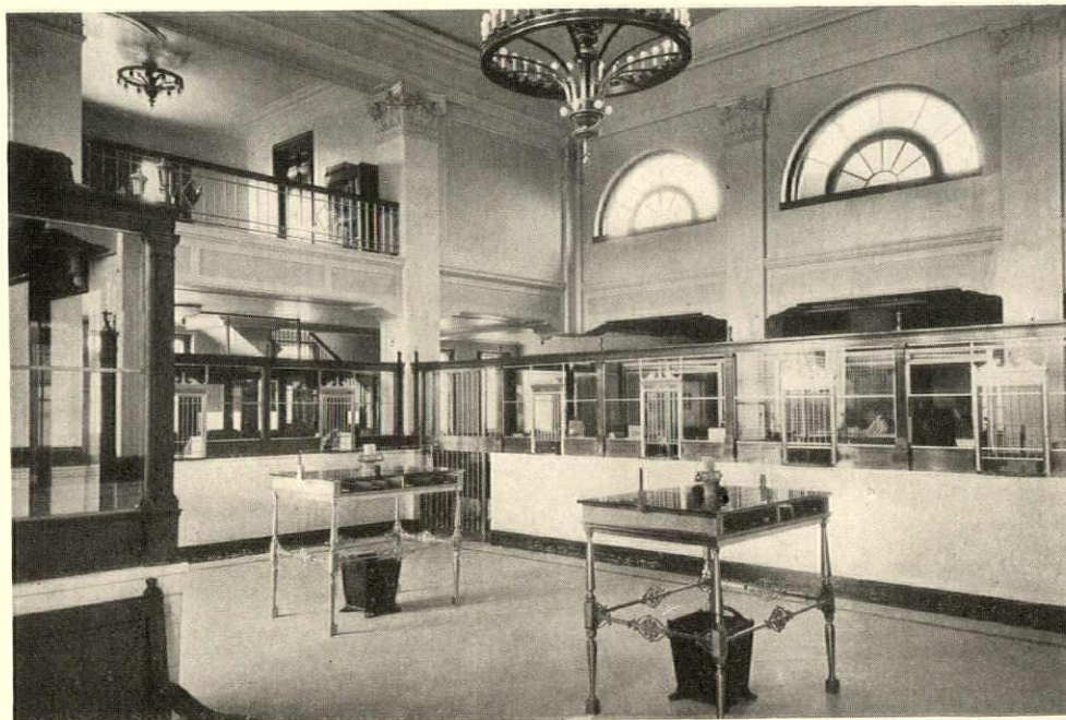
Above, the architect's preliminary perspective of the main banking room. Below, the public space of the main banking room as executed. The wall surfaces, pilasters, and vaulted ceiling are painted an old ivory, the ceiling being of a lighter shade than the walls. The floor is of Tennessee marble, the counter screen being of marble with a maple top screen and bronze wickets
