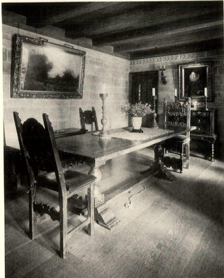
The dining-room. Here limestone was used for the inside facing
