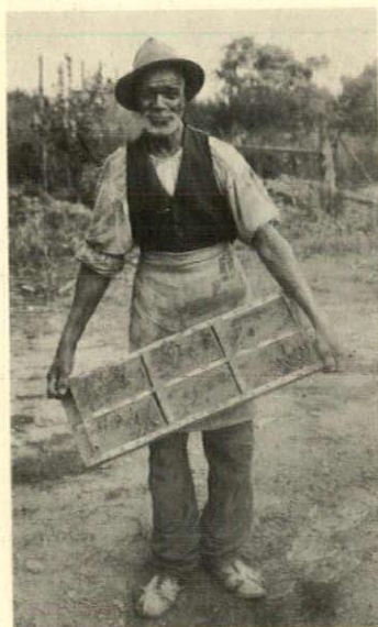
Here's old Rastus carrying away to the drying rooms a mould full of our hand-mades.
