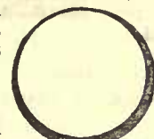
Fig. 230.—Section of a Defective Bell-and-Spigot Pipe.
