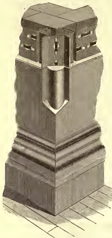
Fig. 5. Perspective showing external angle of brick wall with lathing, furring, screeding, stopped off angle bead, and cement base.
