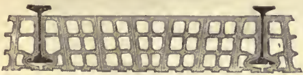
Flat arch between iron beams, with skew-back protecting lower flange of beams.
