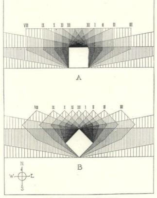
FIG. 1.-SHADOW DIAGRAM OF A CUBE.
