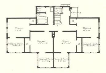
sun. The main entrance is placed at the north of the building to avoid the dust and traffic which would obtain were the entrance placed in the front of the building.
