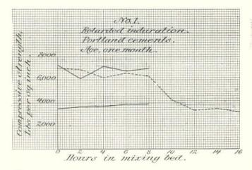
Since it cannot be known, from present information, how a given brand will behave, it would appear prudent to limit the interval to not more than three hours when the cement should be in place after gauging, but generally no anxiety need be felt for Portland cement which is used during the working-day it is mixed.
