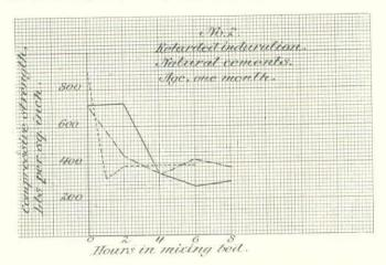
mal strength of the cement when mixed as a plastic mass and immediately used.
