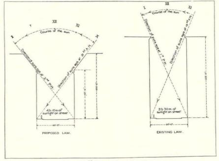
FIG. 12.-HEIGHT OF BUILDINGS. Contrasting the existing law in Massachusetts with the proposed new law. Representing the ross-section of a street running north and south. Latitude of Boston, Mass. Time: March cross-section o and September
