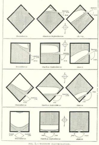
Representing the floor area of an apartment 24' square, illuminated by a single window 3' 6" wide, 8' high, 1' thick, sill 2' above floor, facing north-east, east, southeast and south. Latitude of Boston, Mass.
