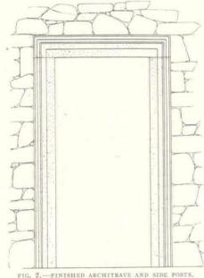
"architrave." The word itself is half Greek and half Latin, and means the "main beam." As this indicates, the architrave was originally the beam, either of wood or stone, which spanned an opening. To strengthen and finish their rough walls at the sides of the opening, and to give a firm attachment for the doors, the
