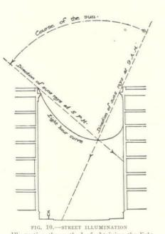
Illustrating the method of obtaining the light curves of the three preceding diagrams. Street running southeast and northwest, looking north-west. Latitude of Boston, Mass. Time: June 21.
