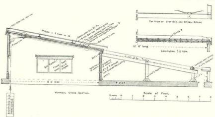
FIG. 5.-DESIGN FOR SMOKE-VENT, WITH SLIDING SHUTTER..
