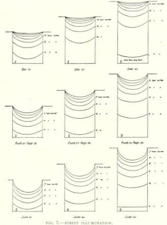
Representing the cross-section of a street running north-and-south. In the left-hand column the height of the buildings is equal to the width of the street; in the central column one and one-half times the width of the street; and in the right-hand column twice the width of the street. Latitude of Boston, Mass.
