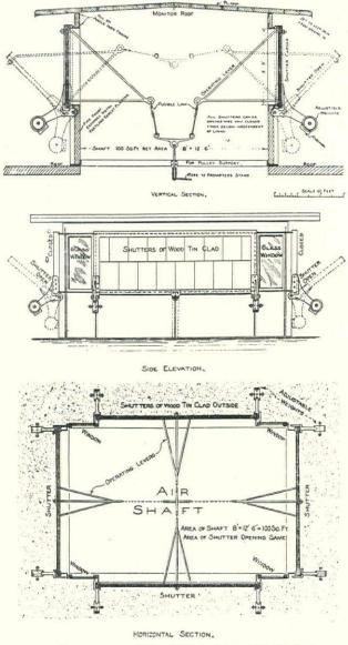
FIG. 3.-DESIGN FOR SMOKE-VENT, WITH HINGED SHUTTERS.
