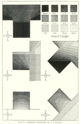
Representing the distribution of sunlight upon the ground surface of a U-court facing north, northeast, east, southeast and south. The height of the court is supposed to be equal to the width and depth. The depth of shade at any point indicates the length of time that point is in shadow, corresponding to the table of tints in the upper right-hand corner. Latitude of Boston, Mass. Time: March and September.
