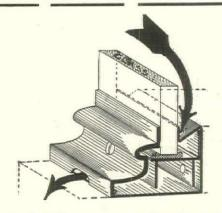
In a store building are pre-eminently a necessity. Kawneer System of Glass Setting provides the only method of draining plate glass that is at once simple, inconspicuous and effective, in a word it is the
