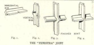
In the "Fenestra" joint, as can be seen above, a small cross slot is made in one of the bars (Fig. 2), only sufficiently large to allow the flange of the other bar (Fig. 1) to pass through it. The moulded portion of the bar (Fig. 2) is then hydraulically pressed out far enough to allow of the moulded portion of the other har (Fig. 1) to pass between it and its flange. other bar (Fig. 1) to pass between it and its flange.
