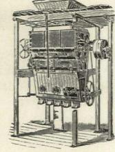
posite directions from one end of the case to the other, keeping it in constant motion and obtaining a perfect mixture.
