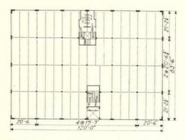
Typical floor plan, giving size of building and position of elevator, stairways and toilet rooms.
