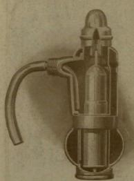
cannot be nullified by inexperienced handling. Just such security is provided by the non-adjustability of the Norwall Siphon Air Valve. It is the most simple, dependable, and extremely sensitive air valve made. It closes instantly against the escape of steam or water; opens instantly to permit the escape of air, and, if flooded, drains instantly through the siphon.
