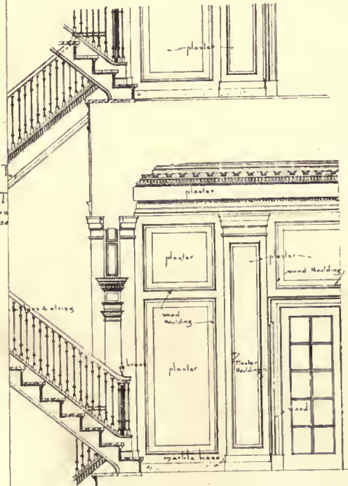
SECTION TYPICAL STAIRCASE
