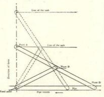
The above diagram shows the position of the levers of the operator when the sash is closed, and when open widest.
