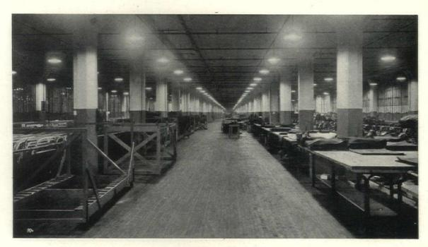
A CLOTHING FACTORY White walls and ceiling lamps mounted high with bowl reflectors, giving good intensity and uniform diffusion on the horizontal working plane. Illumination of vertical surfaces not required in this kind of work.
