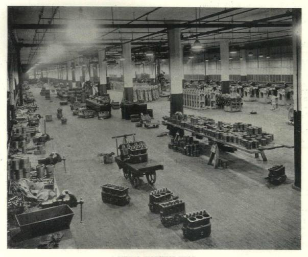
A METAL WORKING SHOP Bench work at the walls, assembling and storage on the floor. White walls and ceiling with lamps in bowl reflectors mounted high. Good light and absence of glare and shadows.
