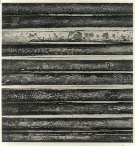
Tests by The Pittsburgh Testing Laboratory, showing the corrosive effect of untreated hot water on six steel and four wrought iron pipes.
