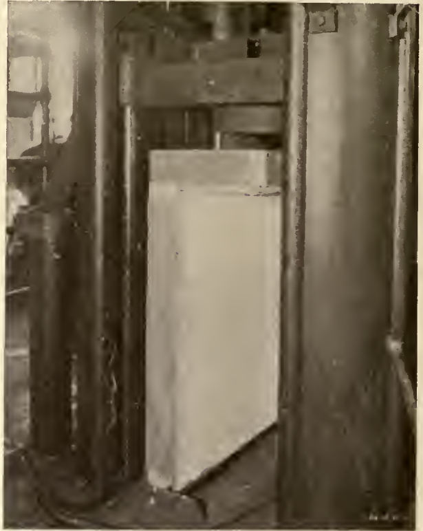
SHOWING TEST SAMPLE SUPPORTED ON END STUD
