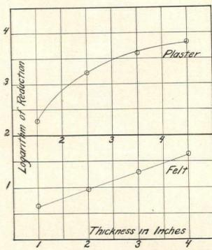
Fig. 2. Average reduction for the whole musical range plotted against the thickness of the partition. Upper curve for plaster on metal lath; lower curve for uncovered hair felt
