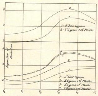
Fig. 4. Curves showing the effects of plastering gypsum tile partitions on the reduction of transmitted sound
