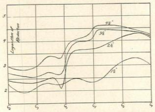
Fig. 1. Reduction of sound transmitted by plaster on metal lath partitions of different thicknesses
