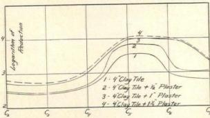
Fig. 5. Reduction of sound transmitted by hollow clay tile partitions
