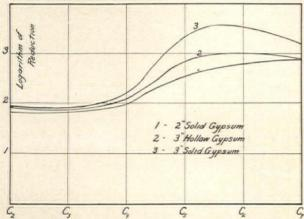
Fig. 3. Reduction of sound transmitted by unplastered gypsum tile partitions
