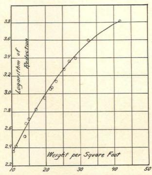
Fig. 6. Average reduction of sound over the whole musical range produced by masonry partitions plotted against the weight per square foot of surface
