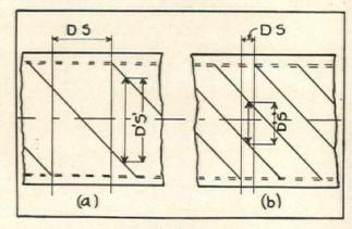
Fig. 3. Effect of Pitch of Spiralling on Torsional Strength
