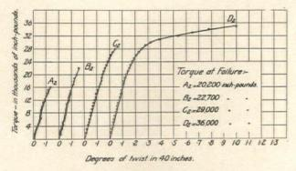
Torque-Twist Curves for 5 x 7 1/2 in. Specimens
