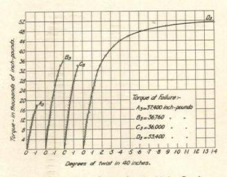
Torque-Twist Curves for 5 x 10 in. Specimens
