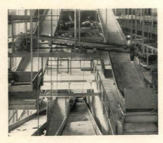
Conveyor belts from floor to floor with separator unit and distributing belts
