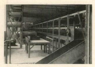
Separator unit, showing the main feed belt with distributing belts on each side
