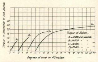
Fig. 4. Torque-Twist Curves for 5 x 5 in. Specimens, Plain and Variously Reinforced
