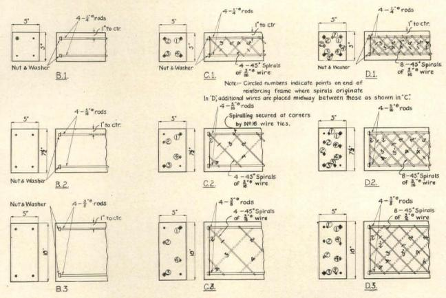
Fig. 1. Rectangular Torsional Specimens of Reinforced Concrete
