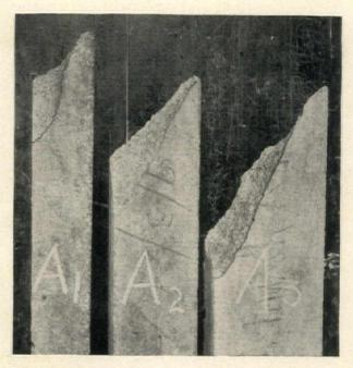
Fig. 2. Torsional Fracture of Rectangular Specimens of Plain Concrete
