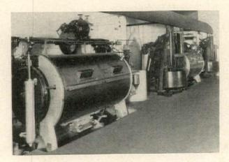
Installation of Direction Motor Driven Washers and Tripod Type of Extractors
