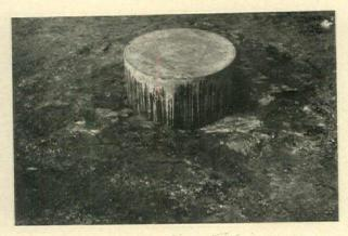
CLOSE-UP VIEWS OF 28" TEST BLOCKS TAKEN AFTER THE TEST LOAD HAD BEEN REMOVED, SHOWING THE CHARACTERISTIC DISTURBANCE OF THE SOIL AT ASSUMED POINT OF ULTIMATE RESISTANCE
