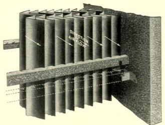
The number of parts and exposed edges are thus reduced. Erection and knocking down for painting are simplified — your clients will value this.
