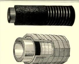
Wyckoff Wood Pipe is built of selected Canadian White Pine in diameters of from 1 to 48 inches. It is durable, economical and quickly laid, and is unaffected by frost or electrolysis. Carries 14 to 20 per cent. more water than metal pipe and will last as long.
