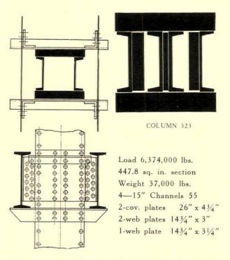
DETAIL OF COLUMN CONNECTION TO DOUBLE GIRDER
