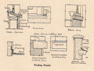
the face and not over the ends. Special attention should be given to the design of gutters and downspouts at returns of porch roofs where overflows will result in discoloration and cracking. A 2-in. strip should be provided at the intersection of walls and sloping roofs and flashing extended up and over it, the stucco being brought down only to the top of the strip.
