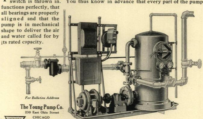
V2 unit equipped for automatic vacuum control, with piping connections made and ready for operation. Piping connections shown in gray tone are to be made by contractor. Suction strainer and check valve at inlet of pump are furnished with unit, as well as companion flanges, bolts and gaskets.
