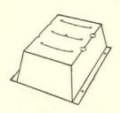
Meyer Tapered Endforms increase the width of the joist and provide a com-pression flange or tee for the supporting beam or girder, and DO NOT in-crease the area of con-crete below the neutral axis.
