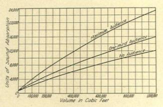
FIG. 6. AMOUNT OF SOUND ABSORBENT NEEDED FOR DIFFERENT SIZED ROOMS
