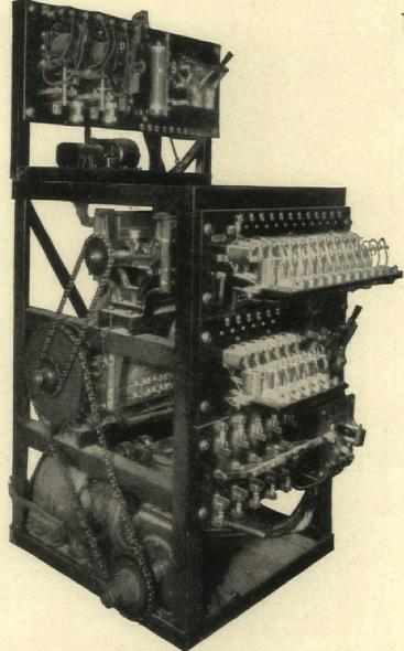
A switch and commutator machine specially designed to operate the signals in the 10 story model building displayed by us at the recent Architectural and Allied Arts Exposition. Machines similar to this operate the signals for a large proportion of elevators now in use throughout the country.
