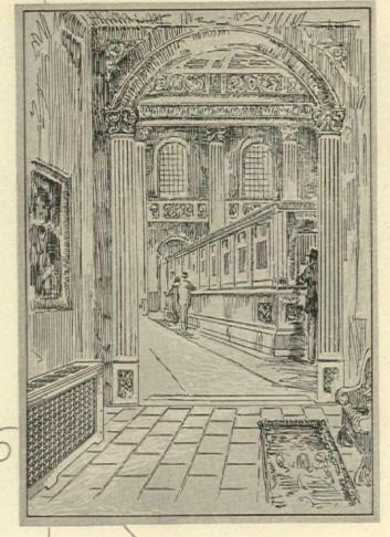
THE use of Radiator Enclosures has greatly increased in the past few years. This demand has brought about a realization that Radiator Enclosures are not only decorative, but add to the efficiency of the heating system by correct heat diffusion when properly constructed.
