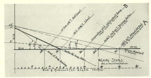
FIGURE 1: Graph analysis of stairways, showing rise, run and pitch. It indicates that many stairways designed by "rule" are dangerous
