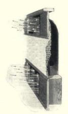
Sectional view of Air-Way Aeriet installed beneath the window and between partitions. Arrows diagram the movement of the cold air entering and varmed air deflected out into the room instead of rising along the walls as with old and obsolete systems.
