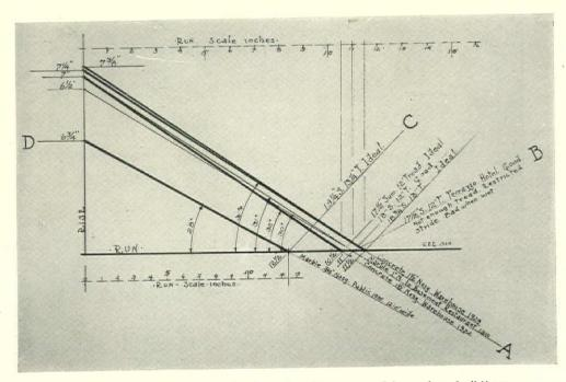
FIGURE 3: Graph analysis of good stairs measured in various buildings
