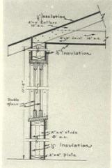
Sound-proof construction of walls and ceilings of studio erected on the stage of the Minneapolis Municipal Auditorium for use at the Eighth Annual Northwest Radio-Electrical Show. Wall studs were staggered. Illustration is by courtesy of the Insulite Company
