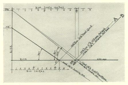
FIGURE 2: Graph of good and bad stairs. That at "B" would be better with a wider tread, giving more pitch to the stair
