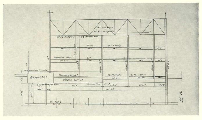
A section showing some of the unusual engineering features of the Daily News Building. Three floors are suspended from a truss, one end of which rests on a column supported by a cantilever girder
