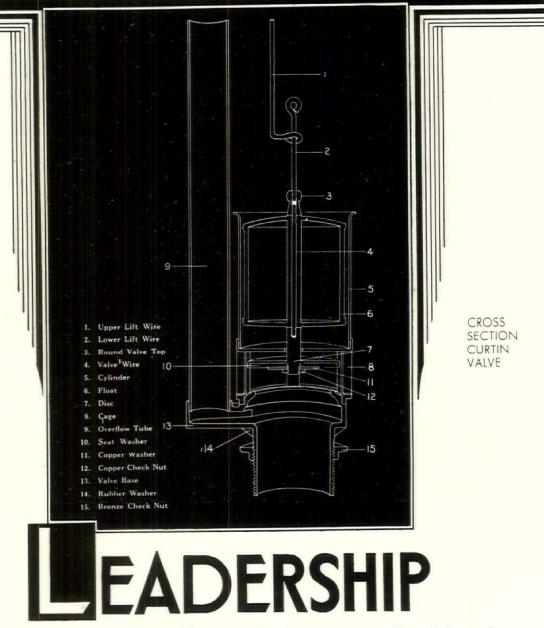
Curtin leadership in the field of fine tank fittings has been effected through the production of long lasting fixtures. Curtin valves and ball cocks, with their bronze and Chase copper tube construction perform their work quietly and most efficiently, without the corrosion and wear that characterize tank fittings of inferior grade.
