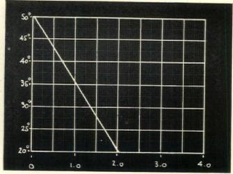
FIGURE 4: Relation between average outside temperature (Fah.) and thickness of insulation required.
