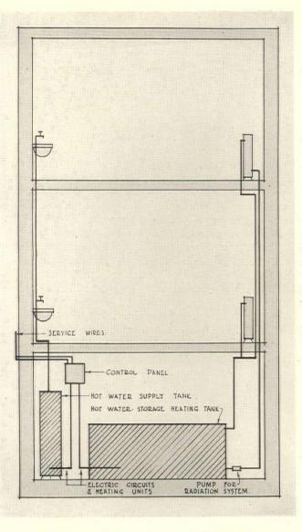
Diagram showing the essential features and typical arrangement of units of an "off peak" electrical heating system
