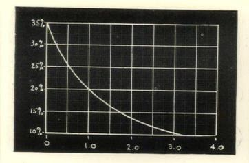
FIGURE 3: Relation between return on investment and thickness of insulation required.
