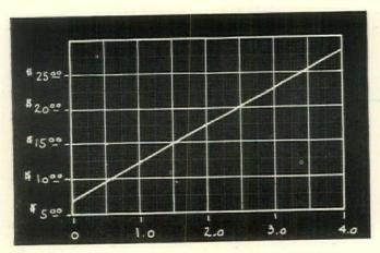
FIGURE 1: Relation between cost of coal and thickness of insulation required.
