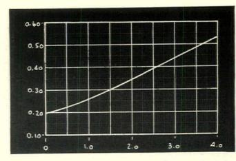
FIGURE 5: Relation between coefficient of transmission of wall and thickness of insulation required.
