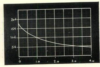
FIGURE 2: Relation between cost of insulation and thickness of insulation required.
