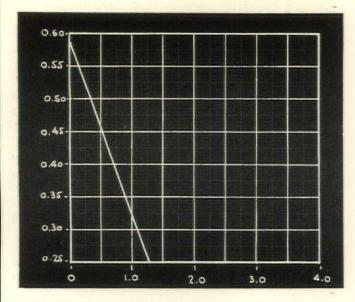
FIGURE 6: Relation between conductivity of insulation and thickness of insulation required.
