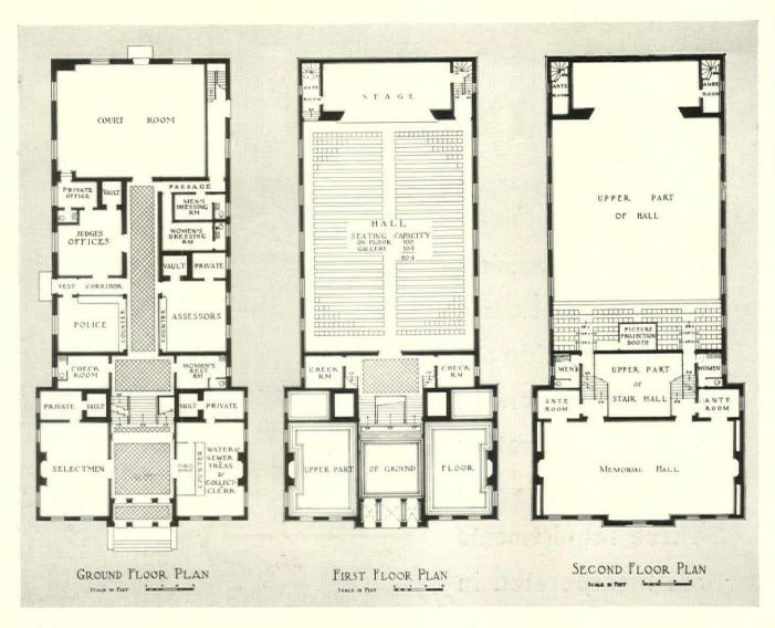
The plans of the Town Hall at Westborough, Mass., show a direct approach to the problem of designing a building to meet the requirements of use and location. The site is one hundred feet wide and flanked by relatively high structures
