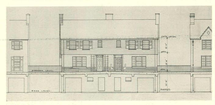
Different levels are provided for automobile and pedestrian traffic as shown by this section looking toward Group C
