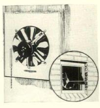
A new type of builtin ventilating fan for residential use has heen announced by the Electrovent Corporation, 5057 Woodward Avenue, Detroit. It is sold complete with a box frame sized to go between standard 16" studding without cutting, being mounted like a window frame. The motor is of a special, brushless type which
