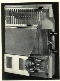
A new heating device called the Electric Aeriet has been placed on the market by the Air-Way Electric Appliance Corp., Toledo, Ohio. It consists of a motor-driven fan which draws the air into the Aeriet, passes it through a specially designed heat element, and projects it into the room. The electric heat unit is a low temperature non-glowing element. It is operated by a threeway switch; one turn
