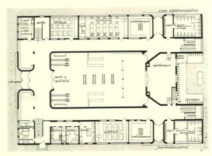
Laboratories, toilet rooms, offices and gymnasium are on the ground floor. Class rooms are arranged on the upper floors. The transverse section indicates a building of utmost structural simplicity
