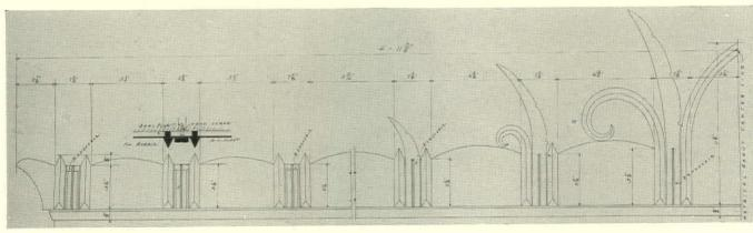
CRESTING over the directory board in the main lobby of the Chrysler Building, New York. The flat members with curved top are cut from sheets and shaped; the short vertical members are bar material cut and shaped; the line between the vertical members is machine engraved; the curved members are hand forged and hand engraved. Assembled partly by welding and partly by chrome nickel screws. Executed by Oscar Bach. William Van Alen, architect
