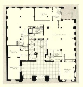
THE GROUND FLOOR PLAN had to make provision for a large number of visitors. The preliminary plan, shown at the top of the page, was faulty in that visitors would not be under full control, and the printing plant was not concentrated. The final plan, shown above, remedied this fault and in addition provided three rooms where exhibits can be held
