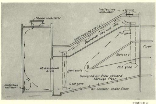
FRONT SEATS COULD NOT BE SOLD in this theatre because defects in the ventilating system made them cold and drafty. An uninsulated roof caused a down draft from the cold attic
