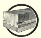
BLOXONEND comes to the job in 8-ft. lengths with small tough blocks of Yellow Pine dovetailed endwise onto base-boards. The endgrain fibres form the wearing surface.
