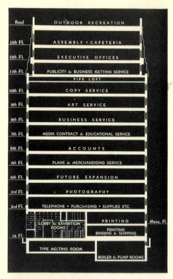
AN ANALYTICAL STUDY was made of the functioning of the organization before any preliminary work was done on plans.
