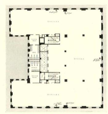
PLAN STUDY COMMENCED with a typical floor. Elevators were placed near the light court, making it easy to handle visitors from a central point. A preliminary study, shown at the top of this page, had too many columns. The final typical plan, above, has fewer columns and the stairs provide interfloor communication from each elevator lobby
