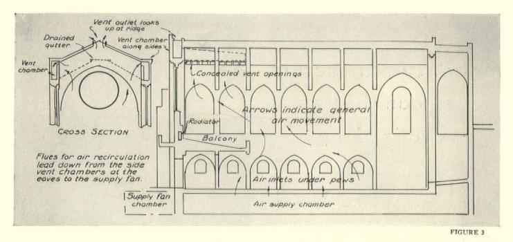
ONLY AN AVIATOR can see the up-looking outlet at the ridge of this church. It is a modification of the ridge vent detailed in Figure 1. This arrangement worked
