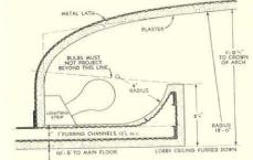
COVELIGHTING of a new type in the ceiling of the entrance lobby, section of which is shown above with photograph at the right. The ceiling and wall surfaces are painted black, except the piers and ceiling recess which are painted white
