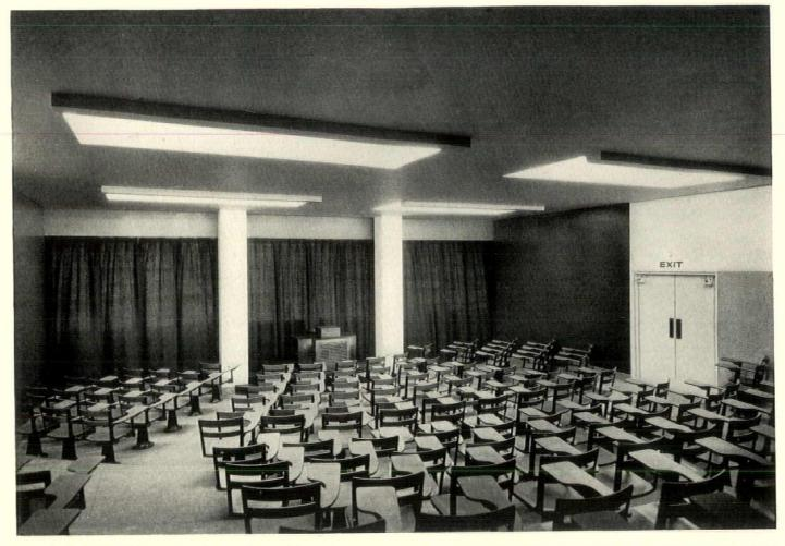
NO GLARE in students' eyes from this system of lighting, whereby diffused light is reflected from rectangular ceiling recesses with strip reflectors partly recessed along the back edge
