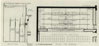
■ SEATING SIX HUNDRED Nichols Intermediate School, Evanston, III. Stage is 22' x 45'; proscenium is 30' x 17', gridiron is 33' above stage. Cost of curtain equipment, \$4,150; stage lighting, \$5,000; stage equipment, \$4,000. Erected in 1929.
