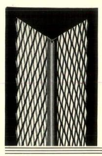
The Plaster is Keyed Right up to the Nose of the Bead >>>•<<<
