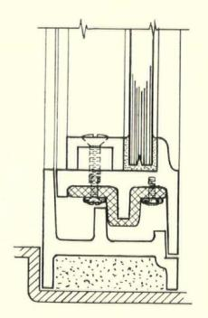
Window openings are closed with "Halco" Casement sash, on the Mooring Tower of the Empire State Building. Note the three-point contact of sash and frame and the air tight seal of solid rubber, shown by the above detail, which is actual size.
