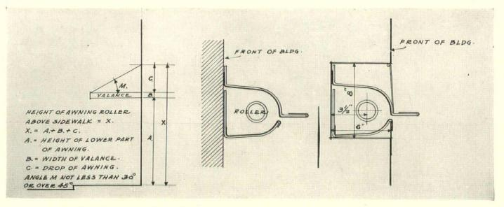
Diagram of height above sidewalk and projection; typical detail of awning boxes on face of wall and recessed
