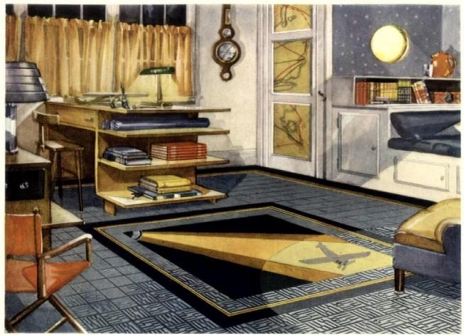
Armstrong's Linoleum, Plain and Embossed (No. 3221), cemented in place over linoleum lining felt, forms the floor for this air-minded room. Insets such as that above can be made up in any design.
