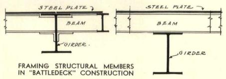
Above left, recommended method of framing beams into girders. . . Above right, framing beams on top of girders
