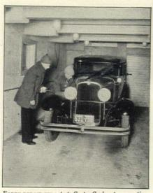
FORTY BELOW ZERO tests Carter Carburetor operation here, thanks to Armstrong's Corkboard on the walls and Cork Covering on the cold lines.
