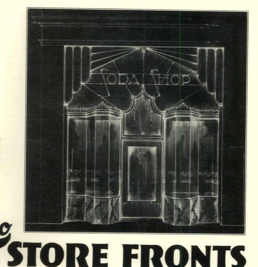
Perspective drawing of Soda Grill in Dempsey Hotel Bldg., Macon, Ga. Desco modernistic Store Fronts, extruded, cast and rolled aluminum are being used for this interesting remodeling job.
