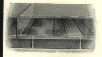
Cheney Flashing Installed— Phantom View Thru-the-Wall
