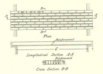
BARS are placed in mortar joints when constructing a simple reinforced brickwork slab
