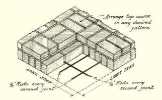
FOR LONG SPANS and heavy loads brickwork slabs, two courses thick and reinforced in two directions, are suitable. The upper course may be laid in a decorative pattern
