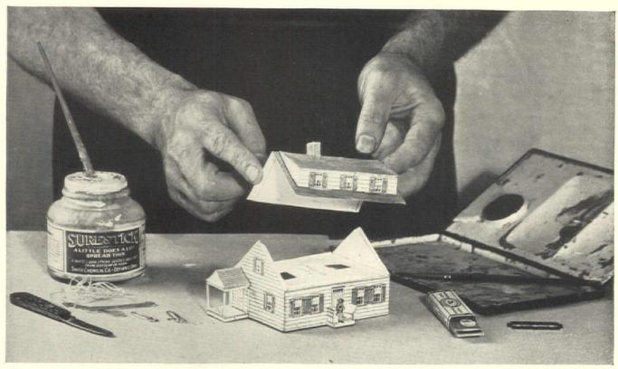
After rendering with water color, assembly is started. Note horizontal bracing
