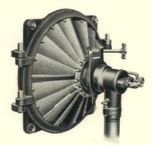
Model "H": Air turbine driven rotary cup burner for heavy duty. multiple burner installation. Air and oil supplied from central fan and pump set. Manual ignition.
