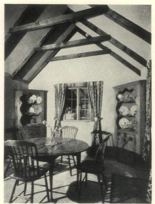
INTERIOR WALLS were finished with a coat of 3/8-inch plaster, applied direct to the cinder blocks, and a coat of paint sprayed on. Plaster board was used for the ceiling with 3" x 4" timbers exposed in the living room and dining room
