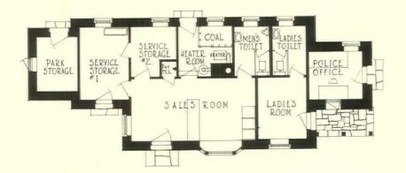
The service station problem of the Westchester, N. Y., park system has been well studied both as to appearance and relation to traffic. The stations are reached by a bypass road paralleling the main highway. The one shown on this page is on the Hutchinson River Parkway. It is built of local stone. Gable ends are shingle and the roof is of slate. Its cost, including pumps, exclusive of grading and paving, was \$15,000
