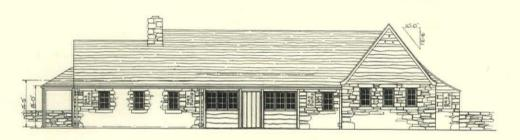
A parkway service station and police office combined. It is located on the Sawmill River Parkway. Exterior is of local stone. Gables are of cedar siding and roof of wood shingles. Interior finished with tile walls, plaster ceiling and cement floor. Note method of recessing pumps. Cost, exclusive of grading and paving, \$21,700
