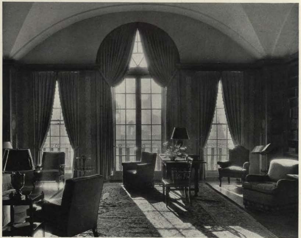
Above: The Lounge. Walls and woodwork painted buff and white. Fireplace, white marble. Fireplace shelf, Levanto marble. Room base, Levanto marble. 18th century wall paintings. At right: The Library. Woodwork, butternut with gold leaf ornament. Plaster ceiling painted white. Floor, cork in two shades of brown. Fireplace on opposite side of room is of pink marble
