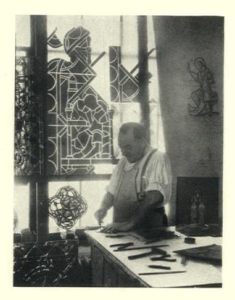
full-size cartoon with a primitive stick of charcoal, is, and always has been, a fundamental necessity of this interesting and inspiring craft. The diamond point, devised as early as the 17th century, and the cutting wheel have replaced the crude, ancient method of drawing a hot iron over the glass and then dipping it in cold water in order to fracture it at an indicated outline.
