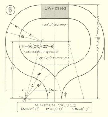
FIGURE 6. A minimum turn-around similar to Figure 5, except for the tangent at landing point. Over-all depth and width of forecourt is increased by the use of the straight landing section, as compared with the preceding plan
