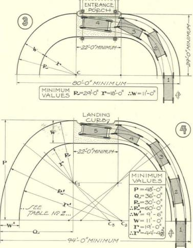
interposed straight landing could extend to infinity and yet the car could *never* become quite parallel with it and snug to the curb without "jockeying" the car into position.
