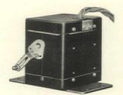
MODUTROL MOTOR. Modulating type. Used in large or small air conditioning systems for modulated control of dampers, louvers or valves. Low voltage.
