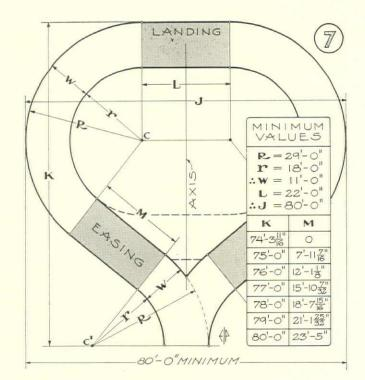
FIGURE 7. Driving is made easier by "easing" tangents at points where direction of curvature is reversed. Inserted table shows that depth K is only slightly increased by extending the easing tangents M. Compare with Figure 6.
