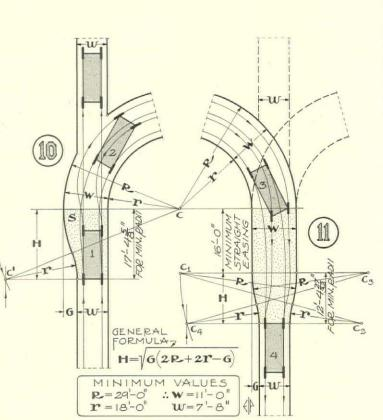
FIGURE 9. A minimum "Y" turn or back-around at a garage entrance, based on simple curves demonstrated in Figure 1. Solid lines show the minimum pavement limits when car enters garage in forward gear. Dotted lines at stem of the "Y" show required extension of the pavement if car first enters the stem and then backs into the garage
