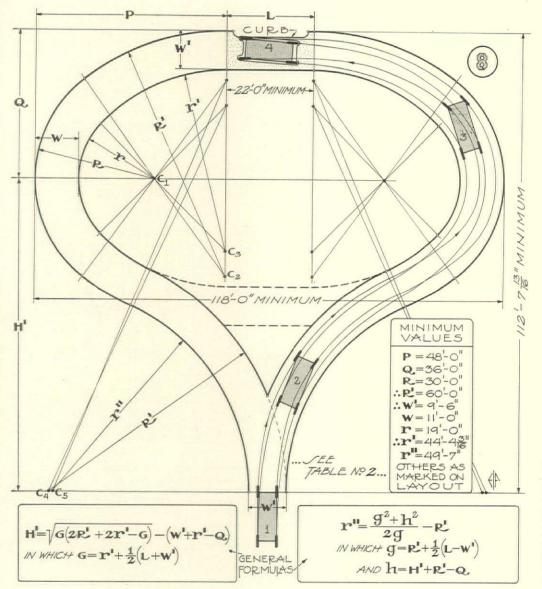
FIGURE 8. A compound curve designed for maximum speed and comfort and considerable driving ease, with a substantially parallel landing at a curb on the main axis. Minimum radii are still used at the ends of the oval, requiring full cramping of the front wheels. Values for larger turn-arounds of this type are given in Table 2
