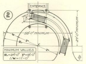
FIGURE 2. On a circular curve, automobiles stop in a raking position with respect to the landing. In an entrance driveway of this type the splay from property line to curb should have no greater radius than the driveway
