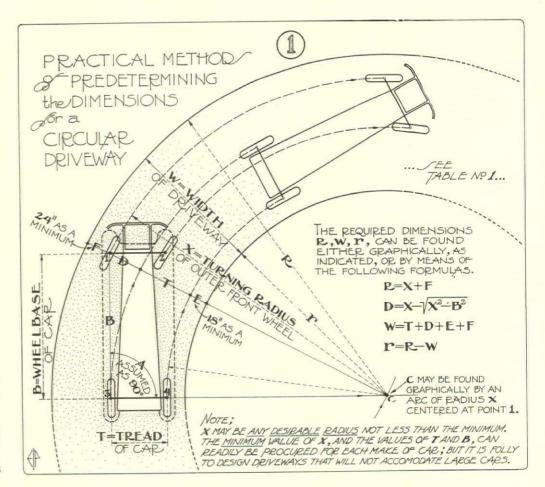
FIGURE 1. The front wheels of an automobile do not pivot about a common point. The rear wheels do not follow the front wheel tracks on curves. Here is shown the geometrical method of plotting the tracks of an automobile on a curve. Table I gives recommended minimum dimensions for circular curves
