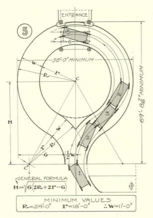
FIGURE 5. A minimum circular turn-around requires sharp turns of the steering wheel from one extreme to the opposite at points of reversal of curvature. The car stops as in Figure 2. Uniform pavement width is permissible even at the point of reversal
