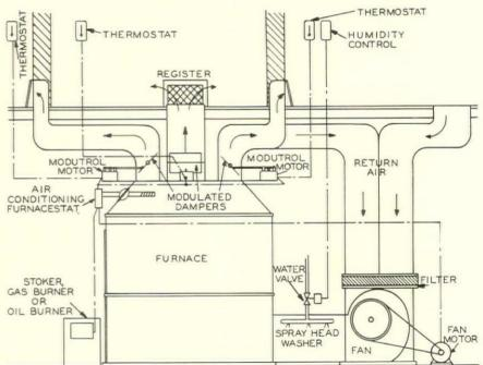
This diagram illustrates the installation of a small but complete air conditioning system. If cooling and humidity apparatus were not included and if air distribution were not to be controlled by dampers, only one centrally located Thermostat would be used — the Modutrol motors and Humidity Control would not be used — and wiring from the Thermostat would run direct to the Air Conditioning Furnacestat.
