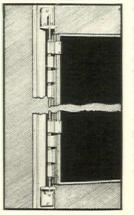
piece of school equipment is in effect a book of blackb o a rds, consisting of four double surface leaves of Hylo plate, bound with metal at the edges and m o u n t e d on two wall brackets by means of the hinge pin. The device gives a writing area
