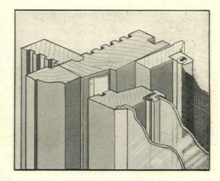
SECTION THROUGH JAMB. Showing Bronze Weatherstrip and Removable Double Glazing. Note special design of sash and frame which prevents sticking and gives two point contact and a third contact with weatherstrip. Note also the wide blind stop and mortar clinch grooves which permit tight joining with the wall in either wood frame or masonry construction.
