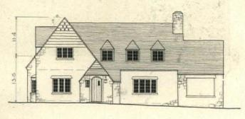
Exterior walls, local limestone ranging in color from cold to warm buff gray. Vertical stone joints filled flush with mortar and surface brushed with a gunny sack. Interior walls, dull ivory, palm-finished plaster. Ceilings, exposed timbers, rough sawn ceiling boards. Floors, oak, random widths. Fireplace facing, common Holland brick. Trim, wormy chestnut. Window sills, kiln run floor tile. 34,500 cubic feet. Cost 53.5 cents per cu. ft. Built 1930
