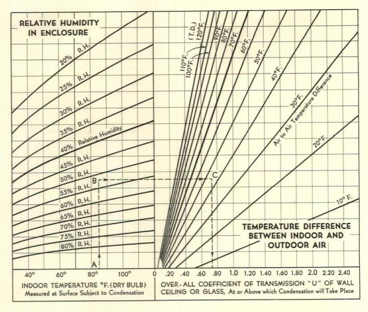
CHART I—CONDENSATION—Curves showing the coefficient of transmission "U" of any construction or glass area at or above which condensation will occur on the innermost surface under given conditions. Use chart as indicated by dotted lines, proceeding from indoor temperature (as at A) to indoor relative humidity (as at B) to temperature difference (as at C—indoor temperature less lowest selected outdoor temperature), to bottom of chart where desired coefficient of transmission will be indicated
