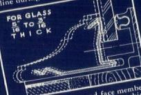
Glass-holding units and face members are self-adjusting to various glass thicknesses without tilting inward or outnesses without tilting inward.
