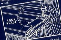
A metal plade inserted in each end of face and locked by pin to rear member is an extra means of securing face in position.
