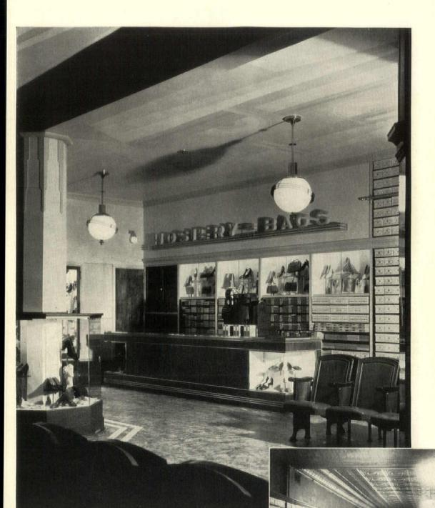
Modernization of this shoe store is typical of possibilities in nearly every city in the country. On the exterior (facing page) an obstructing column was removed from the entrance, show windows were enlarged, the facade faced with Vitrolite and trimmed with aluminum. On the interior the new floor is linoleum; walls and ceilings painted cement plaster; lighting fixtures chromium trimmed with black. Cases and furniture are walnut with chromium trim
