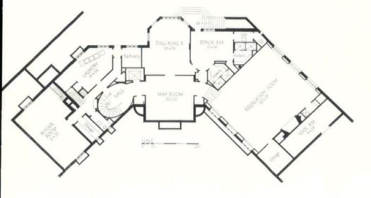
Philip B. Maher, Architect. The house of C. P. Dubbs, Wilmette, III., is built on the crest of a bluff that overlooks the beach of Lake Michigan. Different levels have been utilized in developing the entire basement. The Recreation Room, above, has a ceiling height of twelve feet; the remainder of the area is nine and one-half feet in height
