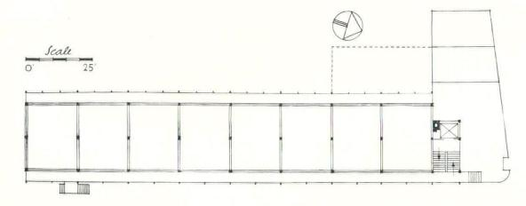
Above: Detail of section through balcony, showing an ingenious form of panel construction. Below: Plan of floors, with 8 identical apartment units divided by double partition walls, with a single lift at the north end. Right: Typical plan of individual apartments. Each unit is a rectangular space, 20 feet, 4 inches wide by 27 feet deep. The exterior of the building is silver-gray metal, yellow brick and glass. Brinkman, Van der Vlught and A. Van Tijen, Architects Section through Balcony
