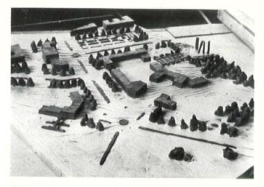
Sketches, thumb-nail perspectives, are used in studying variations in a solution or alternate schemes. Three dimensional studies on built-up contour maps carry the solution still further, as in the preliminary model by William Kittle. Buildings are studied in their relationships to the city plan, as effective units in a great functioning organization
