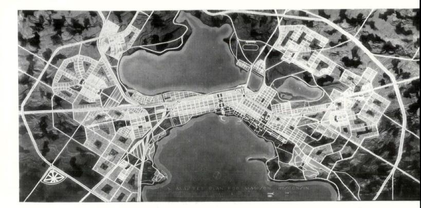
The procedure under Eliel Saarinen is always from the general to the particular, from the controlling factors to the variable. This Master Plan for Madison, Wisconsin, (a project developed by William Kaeser, Architect, at Cranbrook), shows a complete regional traffic system. Such a plan is made after an analysis of present conditions and a synthesis of current trends
