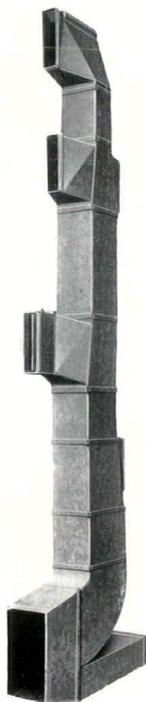
Mechanical equipment in a Reynolds System house is installed in the same manner as in traditional construction. Left: two views of the standard air conduits employed in all Reynolds air conditioning systems. Straight runs, turns and reduction units are kept in stock and assembled on the job with a snap lock joint requiring no solder or screws
