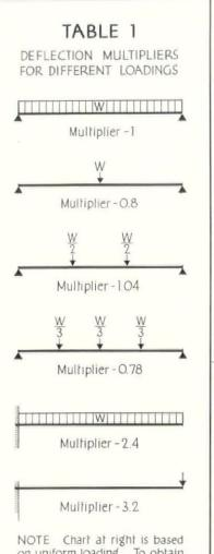
on uniform loading. To obtain true deflection for specific loading, multiply obtained deflectionfrom chart by above multiplier.
