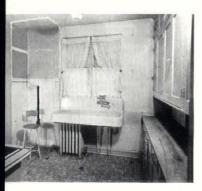
No structural changes. Note the decorative use of ceramic tile, concealed radiator, and wood cuttingtop, the sink and cabinets of metal
