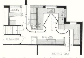
The work area is compact and well integrated. Circulation to house no longer crosses kitchen. The space formerly occupied by kitchen now contains a laundry in addition
