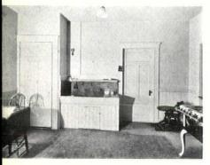
In this modernized kitchen the location of the major equipment was not changed. Individual equipment units were used to effect organization at minimum cost. The wainscot is of composition tileboard, and the floor of linoleum
