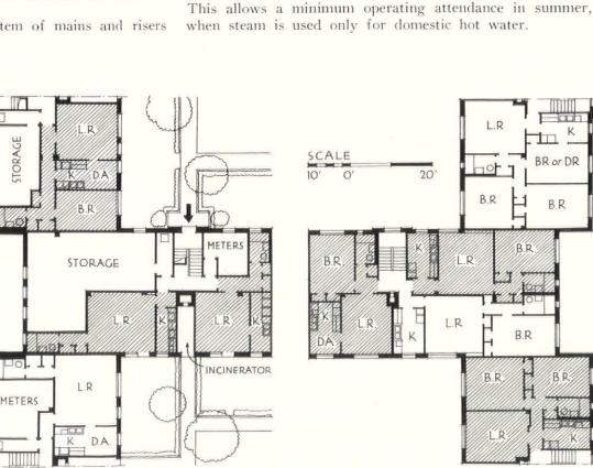
Basement plan showing garden apartments, approaches, and services . . . Typical floor plan (right) showing three-, four- and five-room apartments
