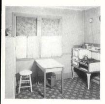
Range and refrigerator have changed places to simplify routine in this kitchen. Note cove base under sink unit, and metal corners protecting synthetic tile wainscot well-appointed small kitchen is not ashamed to be seen or heard, and proper ventilation can eliminate odors.
