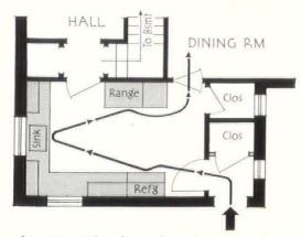
The refrigerator and sink are located in a continuous work surface, permitting easy transference of materials to preparation center. The range with adjacent serving counter is convenient to dining room door. Circulation into the main part of the house still crosses the kitchen but meal preparation routing is much simplified
