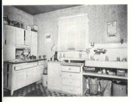
Shifting the sink and adding metal cabinets for adequate storage organized this kitchen. Floor, linoleum; work surfaces, metal; sink, porcelained iron
