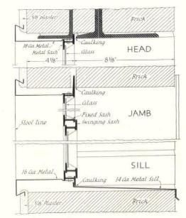
Ingenious and economical window detail, showing metal trim which was delivered fastened to the steel sash.
