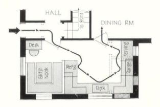
The kitchen routing is simplified, and the traffic into house is kept apart from the working area. A well-lighted dining space has been incorporated
