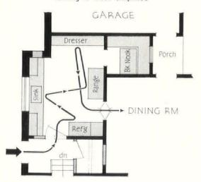
The refrigerator is convenient to the serving center but the door swings introduce mental hazards when using sink or serving center. The former storeroom has been converted into a dining alcove
